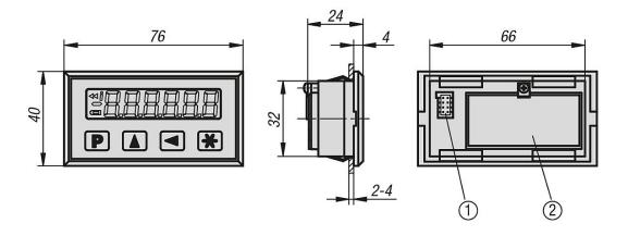
Position indicator, quasi-absolute, network-independent, indicator accuracy 10 µm, small design
