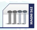
Magni 562 is a chrome-free duplex coating that combines electroplated zinc nickle and hex-chrome-free passivated substrate with an aluminum-rich organic topcoat. A coating that can be engineered to specific coefficient-of-friction needs, Magni 562 is offered with exempt solvents and typically applied to fasteners, including nuts, bolts and other hardware. Magni 562 can be applied via dip-spin or spray application methods.
