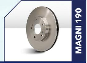
Magni 190 is a high-performance, chrome-free coating – engineered for use on brake rotors and drums – that can be applied on as-cast or machined surfaces. The bright silver appearance provides a refined, premium appearance. This inorganic, metallic film contains proven corrosion inhibitors and lamellar pigments, and offers exceptional cathodic protection in a single thin layer.
